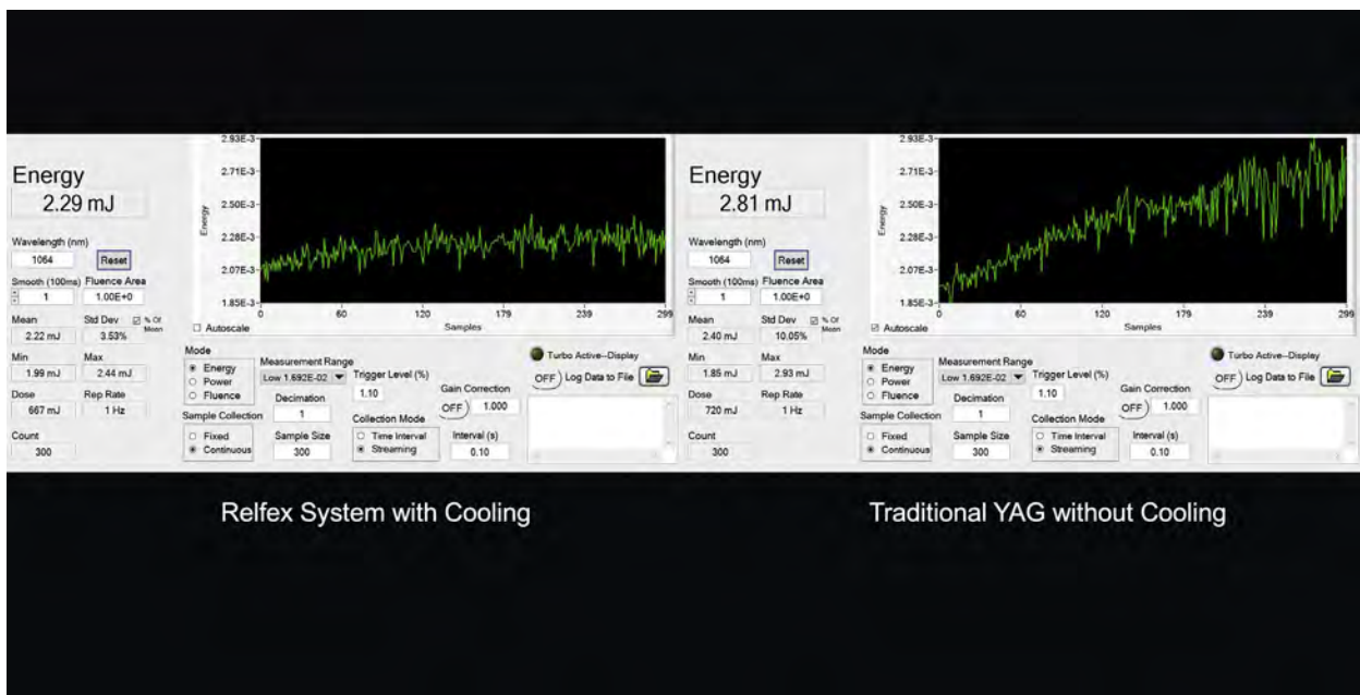
Fig. 10 – Left: Graph demonstrates a stable delivery of energy over hundreds of shots when using active cooling cavity. Right: Graph demonstrates the same when using a passive cooling cavity, the delivery of energy is not stable over hundreds of shots fired. (Poster presented at American Society of Cataract and Refractive Surgery 2019).
