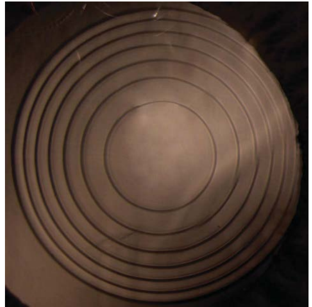
Figure 2. Detail of the lens diffractive trifocal pattern on its anterior optical surface.
